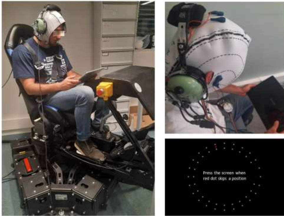
Figure 1: Adapted touchscreen version of vigilance Mackworth Clock test on the motion platform. EEG and alternative EOG electrodes are placed under an aviation headset.
