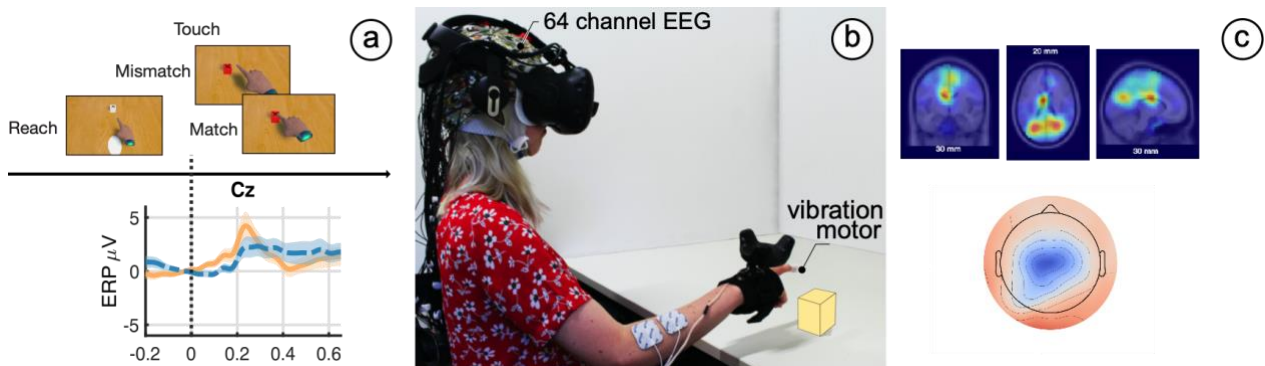
Figure 1. (a) Top: Inside VR task view with example match and glitch, i.e. 'mismatch' trial. Bottom: Grand-average ERP at electrode Cz for mismatch (blue) and match (orange) trials. 0 = collision event. (b) Experimental Setup. (c) Dipole density and scalp map weighted by relevance for classification in the 150-200 ms time window after the collision event.
