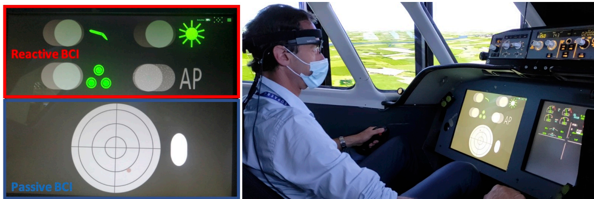
Figure 1: Left: the participants had to perform the checklists with the reactive BCI (in red, upper part of the screen) while their monitoring performance on the radar screen was assessed with the passive BCI (in blue, lower part of the screen). Right: the dual BCI set up in ISAE-SUPAERO flight simulator.
